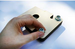
• Put a washer and nut on the threads sticking out the other side. Use a wrench to hold the nut and tighten the machine screw with a screwdriver until snug and small bearings still spin (silver outside of black rubber spins easily but the entire screw/bearing/washer/wood/washer/nut doesn't wiggle around). Do not overtighten.
