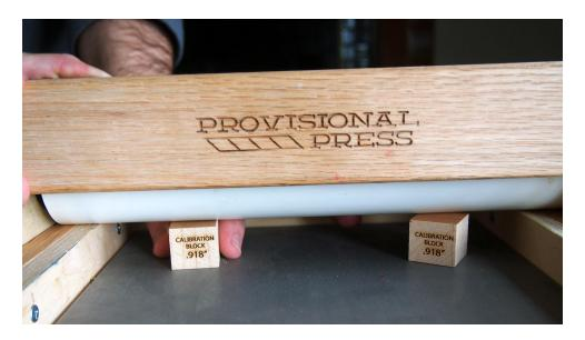
With the press bed (D) and the steel bed plate (or a standard American galley) on the press bed, put two calibration blocks on one side of the press.
